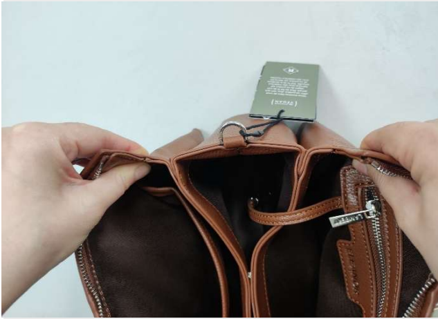
PULL TEST - SEAM SLIPPAGE
